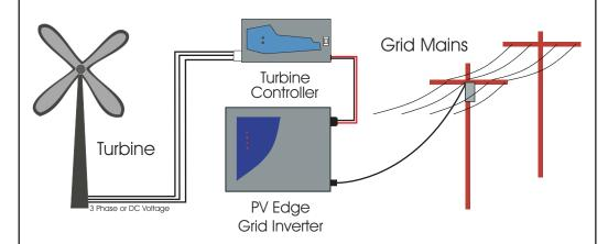
The Latronics Turbine Controller utilises the latest in micro-controller design to deliver a stable and safe supply of power to the grid connect inverter. Designed specifically to integrate with the Latronics PVE1200 Grid Connect Inverter, it allows battery-less grid connection of DC or 3 phase AC wind and water turbines.
