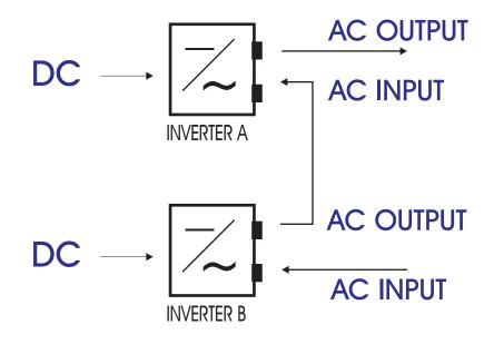
**Dual Inverter Backup Systems** - AC Output will be available as long as Inverter A or Inverter B is operational.
