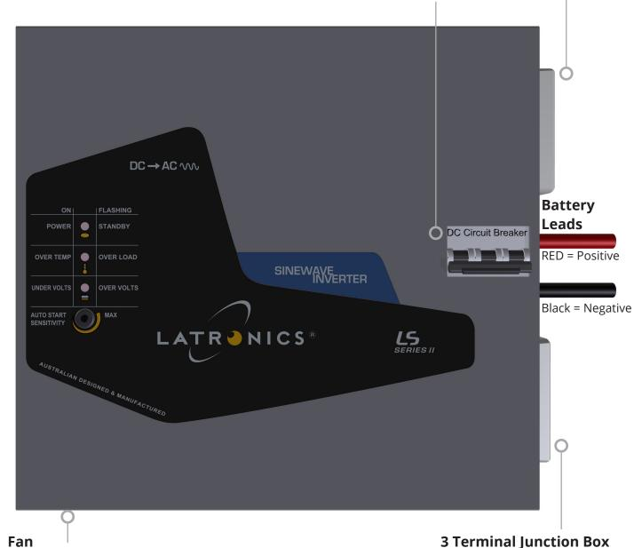
If the temperature inside the inverter reaches preset levels, the dual speed fan will switch on initially in low speed and then into high speed if the temperature continues to increase. Obstruction of the air intake and output will reduce the power rating of the inverter.
